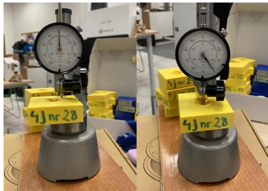
Fig. 16. Measurement of the penetration depth in the examined object using a dial gauge indicator
